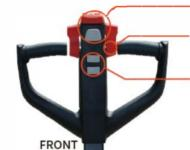
Emergency-reverse & Horn Buttons Dual butterfly-style thumb driving controls
