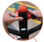
The ability to operate the unit with the titler in the upright position allows working in confined spaces.
